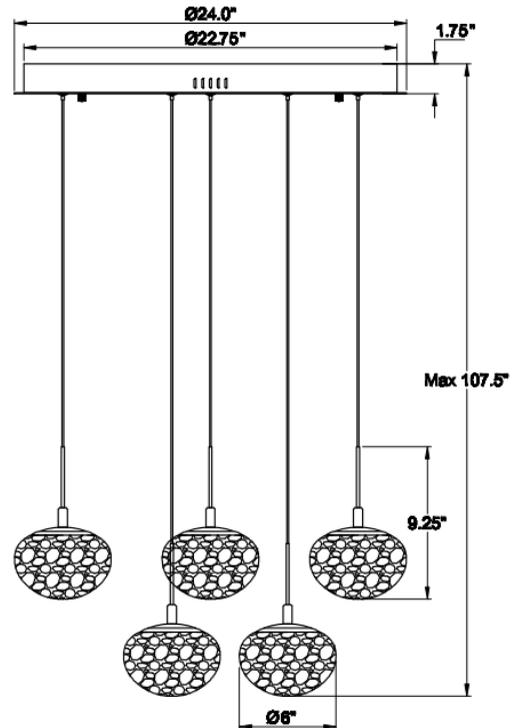
Fixtures weighing 35 lbs. or more must be supported and installed independently of the ceiling outlet (junction) box and require additional support in the ceiling where the fixture is being installed
